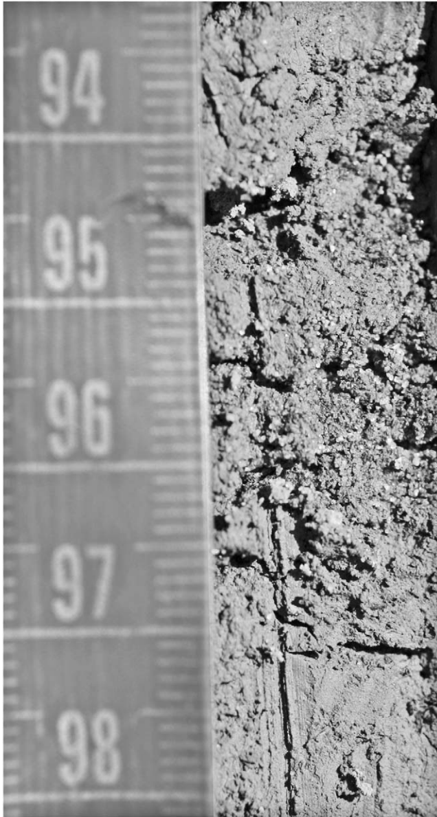
Figure 8. Photograph of bioturbated paleotsunami sand layer (event #3) at site N3 in Neskowin upland flood plain. Grains of quartz-rich beach sand (light) are dispersed in gray silt of alluvial flood plain deposits (dark) by postdepositional bioturbation. Photo is scaled (1-cm intervals) in the field by tape measure.
