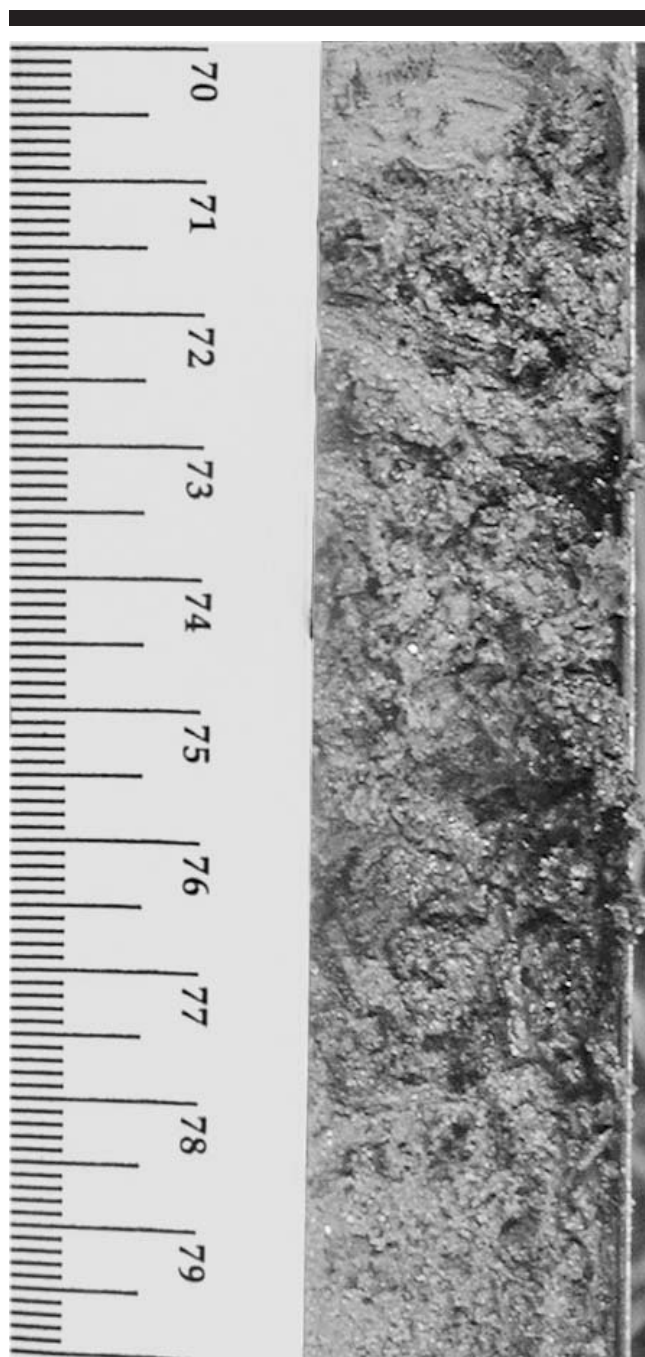
Figure 12. Photograph of #3 paleotsunami debris layer (TDL at 171–179 cm depth) in site B4. Note: Add 100 cm to the 1-m field tape scale. The tsunami debris layer grades upward from fine sand disseminated in silt (179–177 cm depth) to fine sand disseminated in coarse detrital organics (177–171 cm depth).
