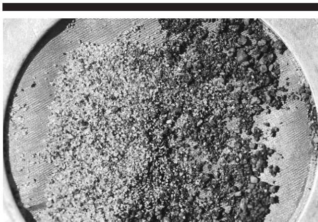
Figure 6. Photograph of two sand types including: (1) target paleotsunami event #3 deposit in site N3 (light: quartz-rich) in photo left, and (2) creek bank deposit in Hawk Creek (dark: lithic-rich) in photo right. Target paleotsunami sand grains are generally well sorted, ranging from ~100–300 μm in diameter. Hawk Creek sediments range from silt in the flood plain to sand and gravel in the creek bed. Mesh screen size is 50 μm in the minisieve (2.5 cm diameter) displaying the two different sand lithologies.
